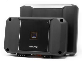
**Convienience and Simplicity** – The R2-A75M features intentional design choices that prioritize convenience and simplicity. All speaker connections are consolidated on one side of the device for easy access, while the amplifier controls have been relocated to the top under a removable plate, allowing for quick adjustments to gain and crossover controls. The amplifier's chassis also includes integrated mounting "feet" to streamline the installation process.
